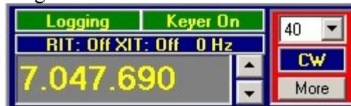
6. You should now see the frequency and mode of the K3 shown in the above Radio section of the main display. Unless you have also connected a keyer and performed the Port Assignment process for it you will see Keyer Idle instead of the Keyer On in the above.
